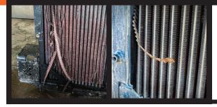
In a recent technical bulletin (SMCS - 1353) published by Caterpillar, the manufacturer announced a design problem with the radiators built and installed on D11 bulldozers: the cooling fins are peeling off the radiator tubes and CAT does not offer a permanent solution to fix the problem. Tubes without fins mean overheating and downtime.
